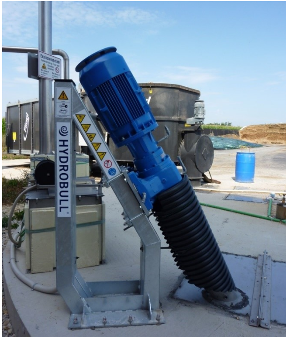
Picture: Streisal Maischebull® / Hydrobull® agitator system for mixing pits and hydrolysis tanks
