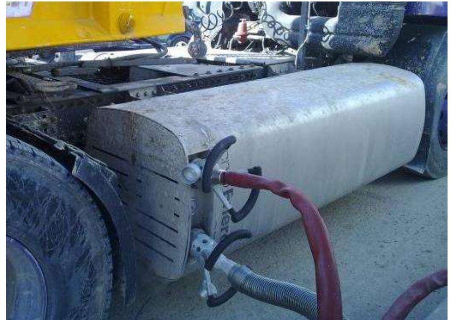
Double hose for filling and venting, high working pressure, 18 bar ( Indox ) (MB to adopt 7-10 bar shortly)
