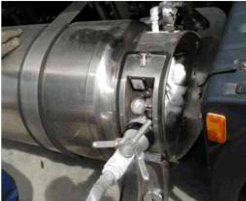
Single hose filling, low working pressure, 7-10 bar ( Chart )
